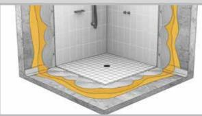
Under tiling waterproofing membrane
