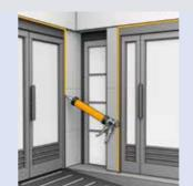
Professional Sealant for Window / Door Perimeter Sealing
